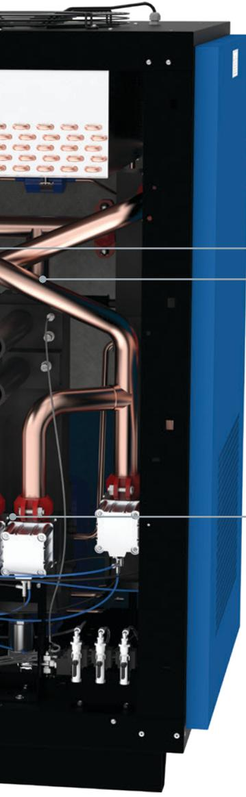
**DRYING:** With only 15% of the of the moisture remaining, the air now enters the sub zero dryer heat exchanger where it is cooled and dried to -20°C (-4°F) PDP. The removed moisture begins to form a thin layer of frost on the inner walls of the heat exchanger.
